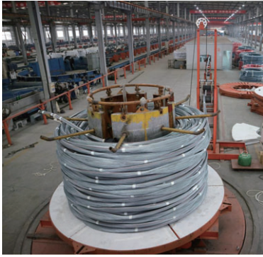
Coiled suspension cables at our Xitang production facility ready for packaging and delivery
