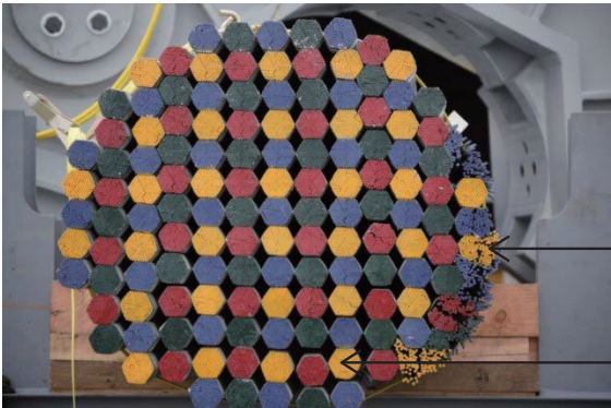
Cross section of a main cable using suspension cable produced by us
