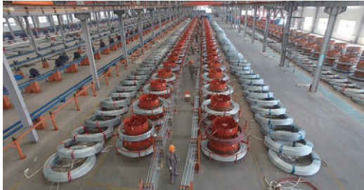
Suspension cables being fabricated at our Xitang production facility
