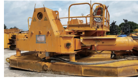
Casing Oscillator (磨樁機)
