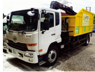
8 Grab tippers Remaining useful life: 0-4.6 years Average remaining useful life: 1.6 years Average actual number of years used: 5.1 years
