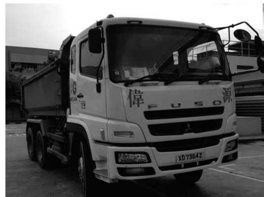
Tipper lorry for transporting loose materials
