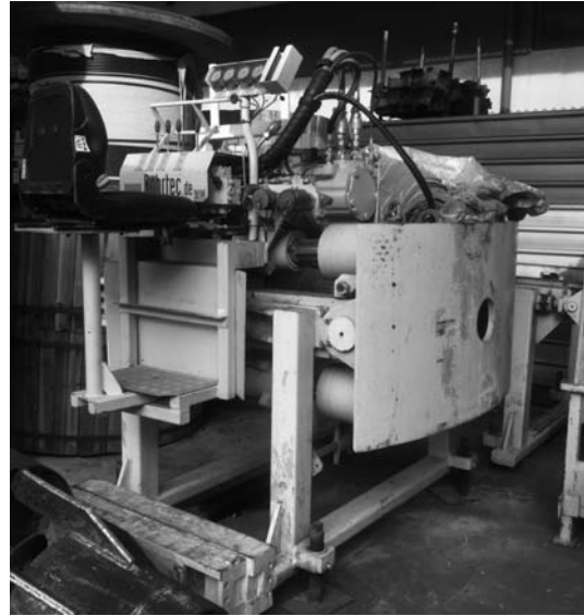
Auger boring machine for pipe jacking
