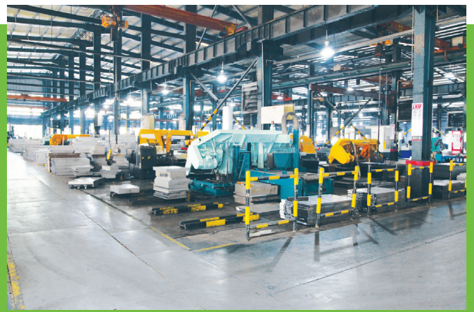
於切割區，鋼材鍛件會被切割成粗形之後才進行加工 At the cutting area, steel blocks are sawed and cut into rough shape before undergoing the rough machining
