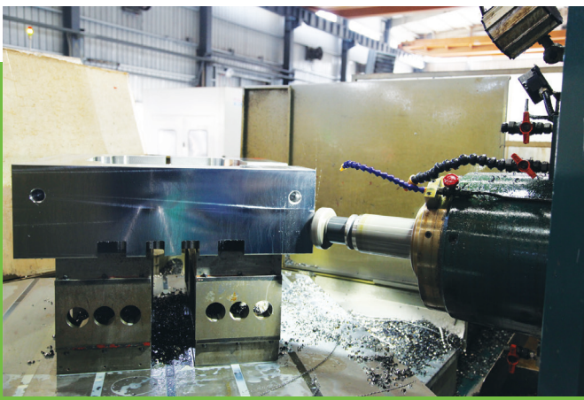
加工中心正為一件大型非標模架進行加工 A CNC machining centre is processing the machining for a large size custom-made mould base
