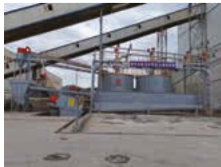
System for aggregates separation with slurry water reuse 砂石分離漿水回用系統
