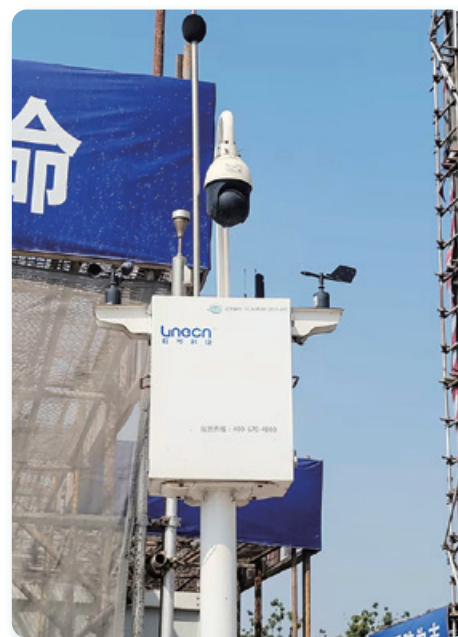
Noise dosimeters are installed at construction site to monitor noise level. Meter reading is recorded few times a day at random intervals serving as random inspections.
