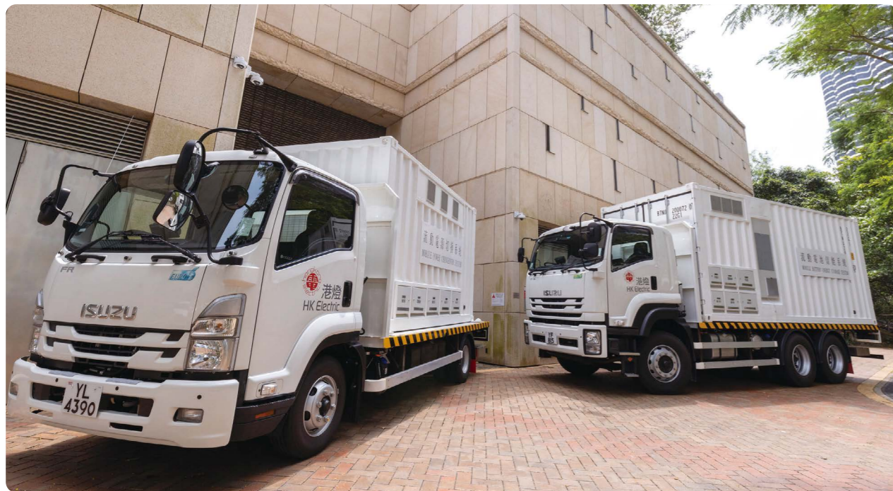
The green mobile electricity supply system, comprising an energy storage truck (right) and a power changeover truck (left), provides uninterrupted temporary relief when normal power is not available.
