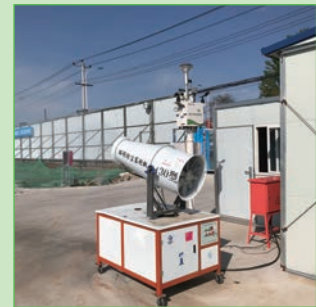
Dust Monitoring and Dust Suppression Equipment
