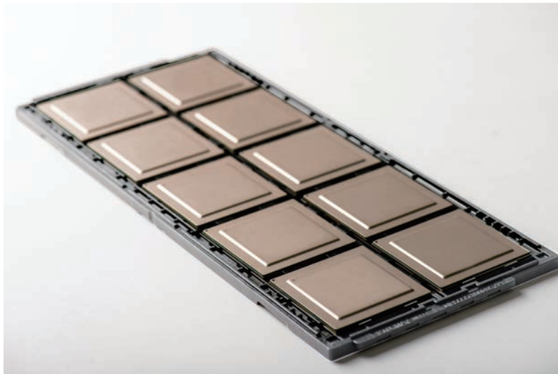
Bakeable JEDEC tray with pocket size of 55mm x 55mm for holding BGA device
