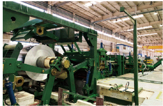
Key technology and equipment development of 2,800mm aluminum strip bending and straightening unit
