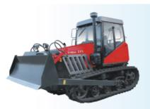
The walking device is a crawler type, mainly used for pulling and driving various supporting equipment, agricultural machinery for completing agricultural operations, earthwork operations and transportation operations. The Company's crawler tractor products have better soil adhesion, suitable for wet soil and soft ground.
